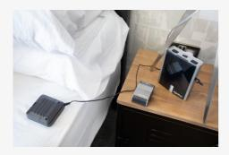
This is a Universal Transmitter attached to a vibrating pillow pad, enabling various transmitters to wake a person whilst in bed.
