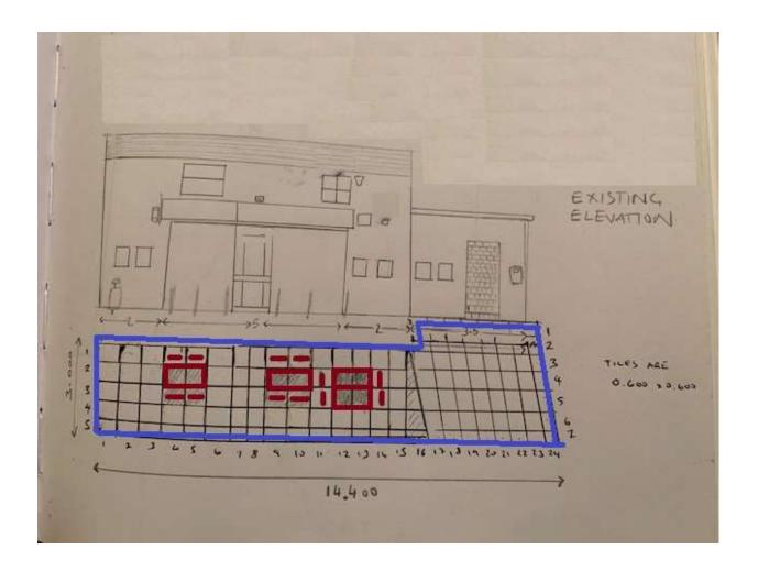
In the above drawing the length of the front of the building is 14.400 m with a depth of 3.000 m from the front. For ease I have drawn out the floor slabs to help you carry out your due diligence.  $5 (5 \times 0.600 = 3 \text{m})$  slabs by  $24 (24 \times 0.600 = 14.4 \text{m})$ .
