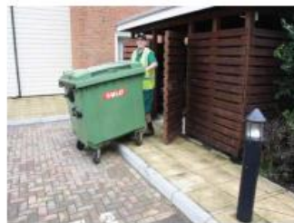
Bin store adjacent to parking space which is not acceptable any parked vehicle will block access to the bin
