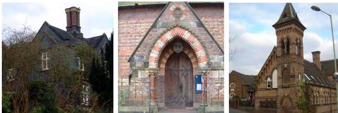
Blue bricks were used for houses as well as public buildings for example 10, Madeley Road, Ironbridge, (left). Polychromatic brickwork acted as a showcase for the local brick trade as seen at Jackfield Church, (centre), and the Wesleyan Infant's School, Madeley Wood, (right).
